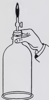
FIG. 24.—Bell Jar of Hydrogen, showing its Inflammability, Lightness, and Diffusibility.
